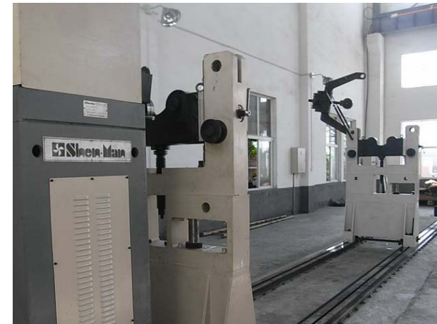
Dynamic balancing machine Length 12m / Max.loading 50T
