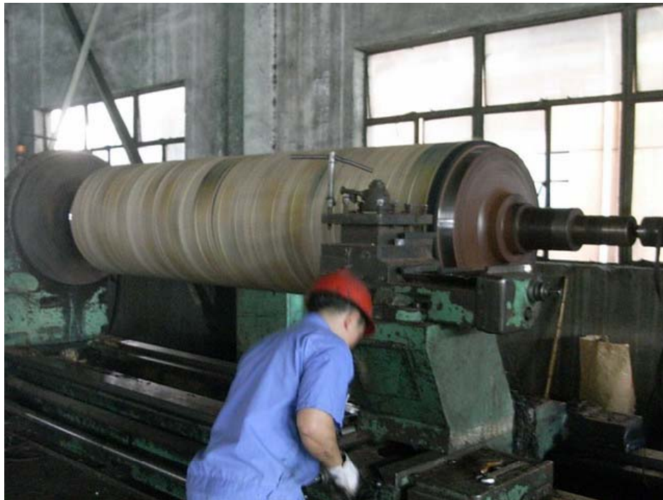
CNC grinding machine Dia.2m x Length 12m
