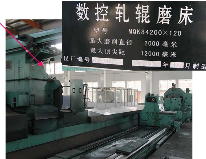
CNC grinding machine Dia.2m x Length 12m
