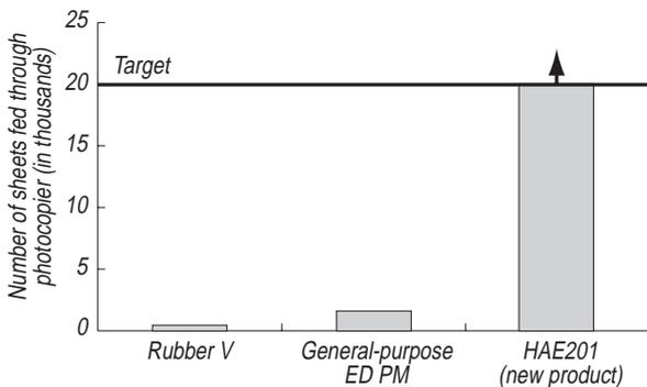
**Fig. 8 - Roller lifetimes when the rollers are used to feed lower-quality plain paper**
