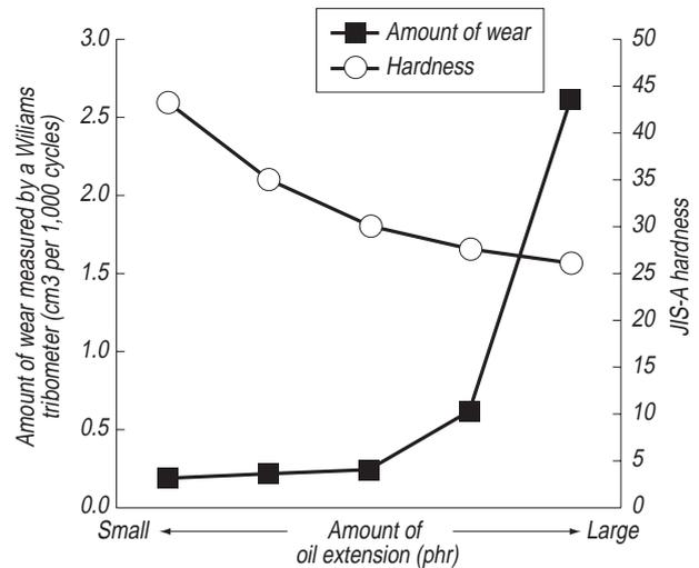
Fig. 6 - Relationship between oil extension and wear resistance/hardness
