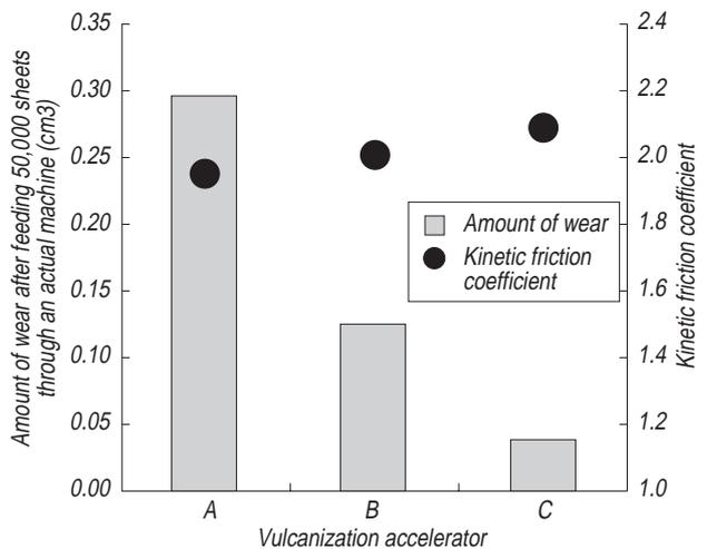
Fig. 7 - Relationship between vulcanization accelerators and wear resistance
