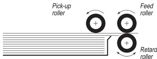
The retard roller is driven in the reverse direction and is equipped with a torque limiter.
