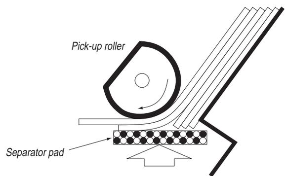
**Fig. 9 - Separator-pad-type separator mechanism**
