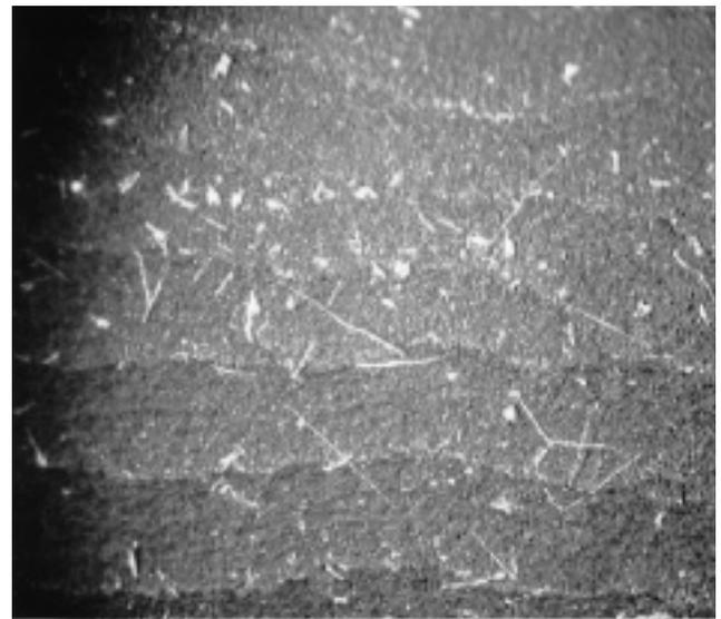
Fig. 4 - Roller surface after feeding the paper made in country A
