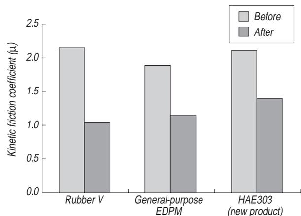
Fig. 12 - Change of  $\mu$  after feeding 2,000 sheets of coated paper A
