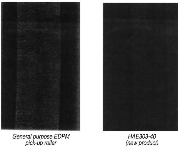
Fig. 11 - Results of printing in the pick-up roller contact region
