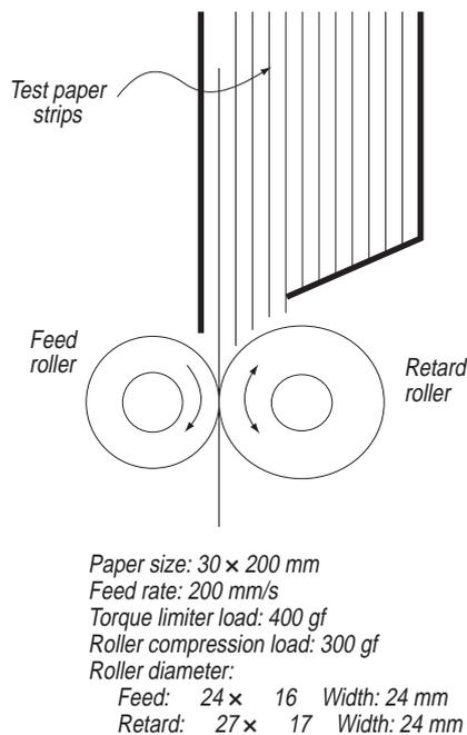
Fig. 2 - Retard roller accelerated paper feed test apparatus
