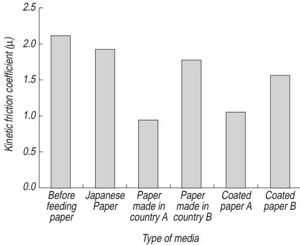
Fig. 1 - Changes in roller  $\mu$  with various types of media
