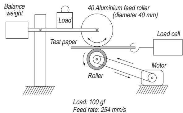
Fig. 3 - Friction coefficient measuring apparatus
